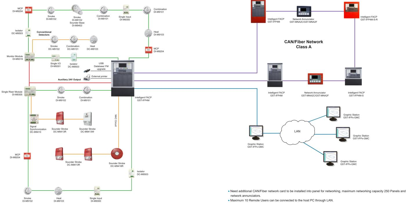
• Maximum output of Panel NAC+ Auxiliary output is 2.5A
